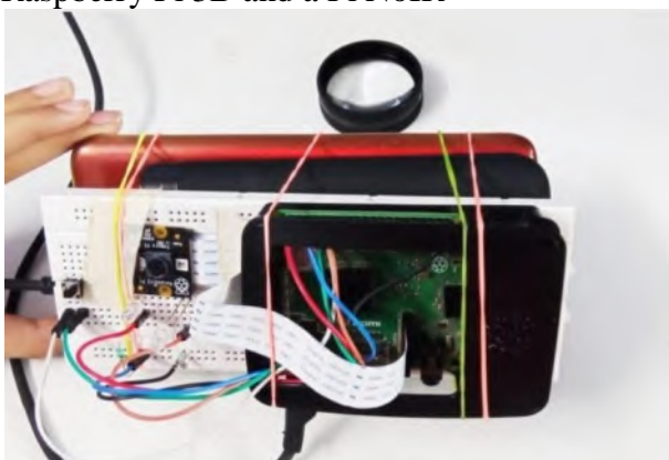
Fig. 8. Handheld build of the fundus camera
